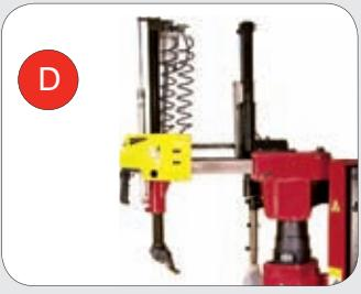
**(EN)** **VERTICAL POST:** Helicoidal automatic swing arm configuration complete with pneumatic control of the working arm. The horizontal head is equipped with triple regulation system for easy maintenance, double locking system and with rollers to improve its movement fluidity.
