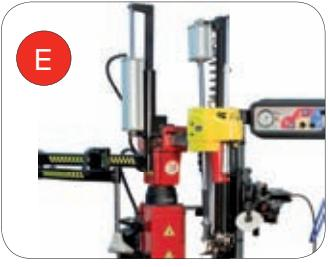
**(EN)** **BEAD PRESSING DEVICE IPH:** New standard supplied independent floating bead presser, integrated in the vertical post, which helps the operator to mount and demount particularly tough or low profile tyres such as «Run-Flat». The bead pressing tool height is easily adjustable for reverse rims handling.
