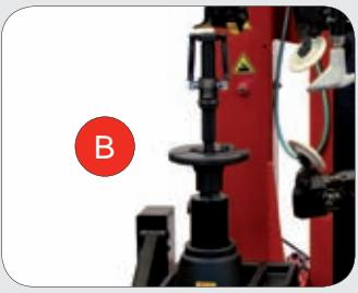
**(EN)** **UNIVERSAL WHEEL LOCKING SYSTEM:** Standard with manual wheel locking system equipped with removable central fixing shaft able to lock rims from 12" to 30". Available optional clamping accessories for non-standard rim shapes. Available on demand the variant with central pneumatic locking system.
