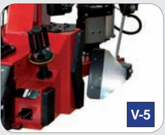
**(EN)** **TRADITIONAL BEAD BREAKING (OPTIONAL):** To be factory installed and with bead breaking blade, it features a double acting bead cylinder and it is specifically conceived to handle mainly steel rims: max rim diameter 17" and max wheel width 320 mm (12,5"). Only for versions with Motoinverter.
