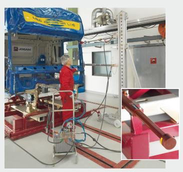
The JOSAM cab bench works together with our aluminium straightening towers and extra accessories related to pulling and pressing.
