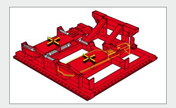
JOSAM cab bench consists of a rigid base which is anchored to I-beams embedded in the workshop floor or floor anchoring drilled into an existing floor (JOATP151). Even a severely damaged cab can be mounted thanks to the movable jig fixtures. The cab floor structure is then hydraulically straightened with moveable 10 ton cylinders located within the bench.
