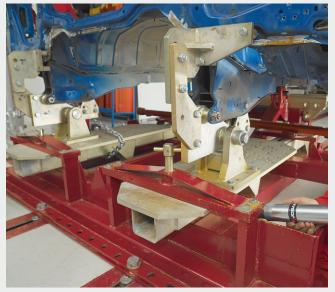
The four mounting points of the damaged cab are anchored to the bench by means of specially designed adapter sets for each cab model. Badly displaced front mounting points are held and pressed into the correct position by using a hydraulic cylinder and moveable jig members. Locating pins are used to guide the mounting points into the correct position.
