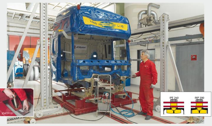
The JOSAM cab bench is a strong and stable aligning jig which simplifies cab repair. Moveable mounting points make it easier to mount even severely damaged cabs. The base of the cab is pushed and pulled hydraulically into its correct position.
